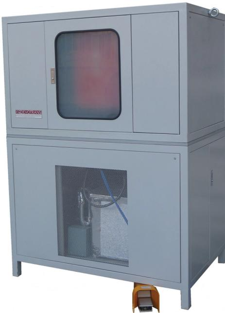
This machine is mainly applied in testing the thermal resistance properties of insulation materials.
